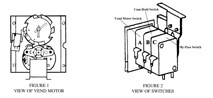
See Vend Motor and cluster switches in stand-by position Figures 1 and 2. Arm of Vend Motor Switch A is in cam notch - Figure 2. Arm of Cam-Hold Switch B is on top of cam - Figure 2. Arm of By-Pass Switch C is on top of cam - Figure 2.
